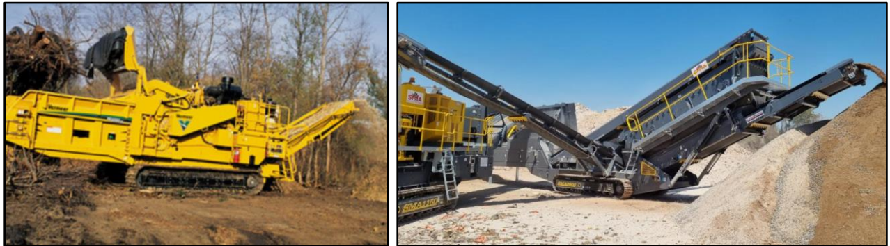
Figure 8: Example biomass grinding and screening mobile plant
