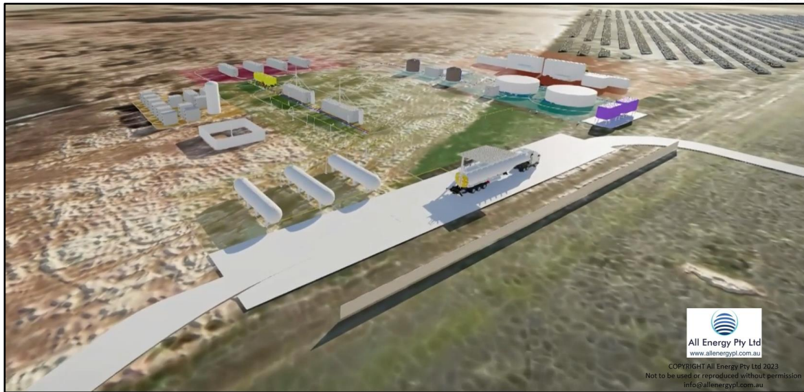
Figure 11: 3D preliminary layout of a 3000 tonne per annum anhydrous ammonia plant using energy from waste and solar.
