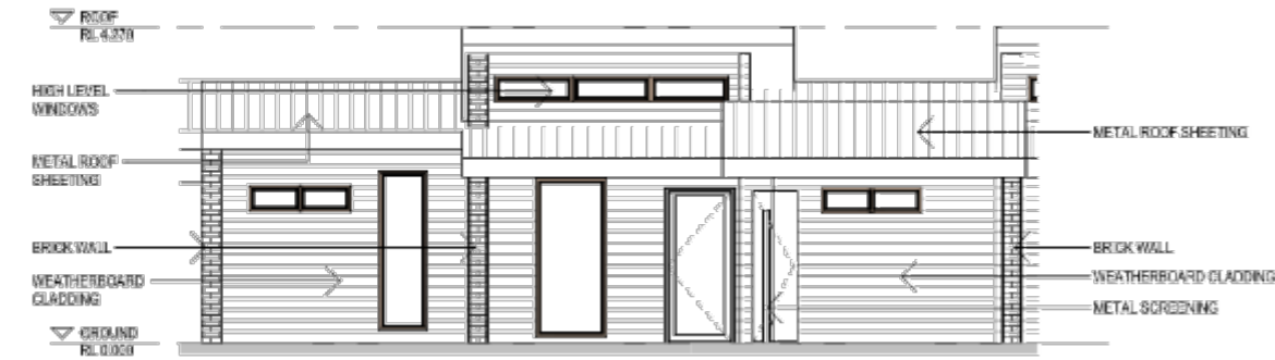
1 TYPICAL 2 BED UNIT SOUTH ELEVATION 190 1:100
