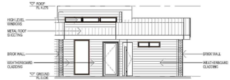
4 TYPICAL 1 BED UNIT SOUTH ELEVATION 190 1:100
